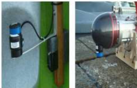
Figure 6. Fixed transponder (left) and acoustic modem/ranging device on the Medusa nose cone (right).
